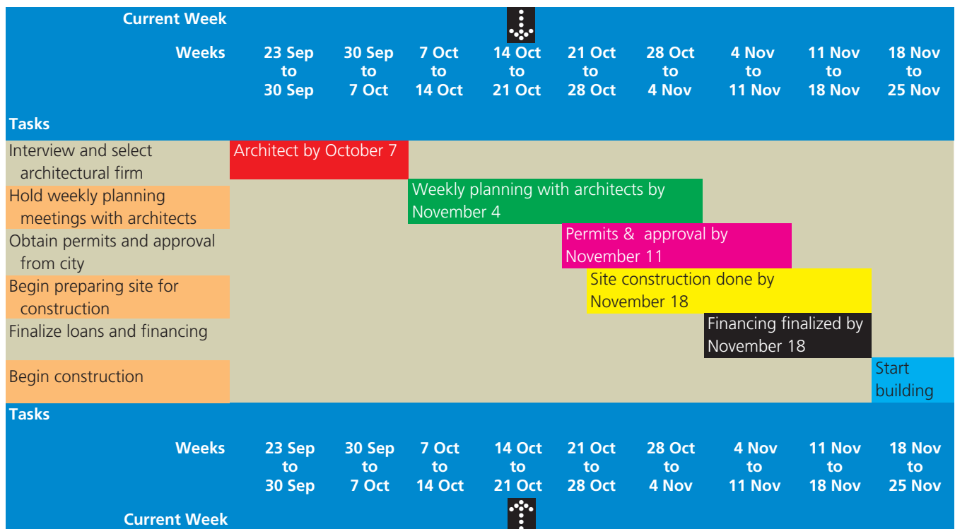
Gantt Chart for Starting Construction on a New Headquarters
